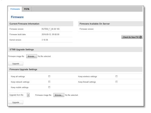
**STM8 Firmware** –it is responsible for sleep mode functionality and signal strength leds.
