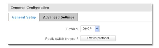
You can switch between the Static or DHCP protocol by selecting the protocol that you want to use and then pressing **Switch Protocol**.
