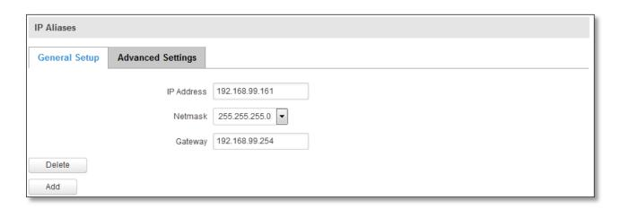
As you can see, the configuration is very similar to the static protocol; only in the example a 99th subnet is defined. Now if some device has an IP in the 99 subnet (192.168.99.xxx) and the subnets gateway metric is "higher" and the device is trying to reach the internet it will reroute it's traffic not to the gateway that is defined in common configurations but through the one that is specified in IP aliases.
