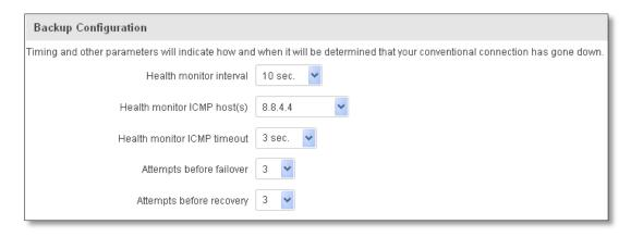
The majority of the options consist of timing and other important parameters that help determine the health of your primary connection. Regular health checks are constantly performed in the form of ICMP packets (Pings) on your
