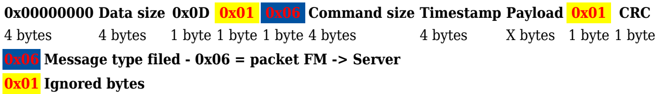
Figure 2. Structure of Codec 13 messages
