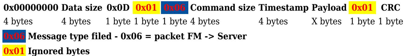
Figure 2. Structure of Codec 13 messages
